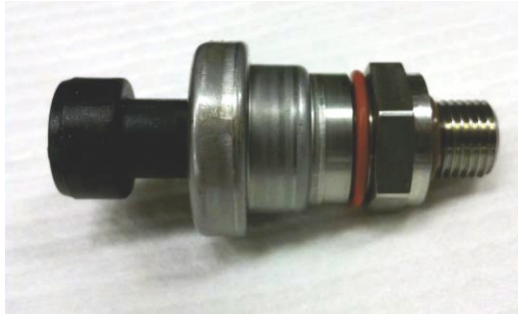
Figure A. 3/4" hex head–transducer identified for replacement
