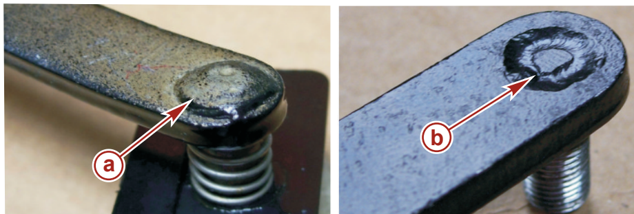
a - A good weld will appear, or feel, as a raised bump directly below the stud on the bottom side of the shift link
